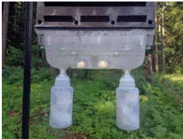
Obrázok 8. Upravená zberná nádoba s nosičmi entomopato- génnej huby Figure 8. Modified collection container of pheromone trap with entomopathogenic fungus carriers.
