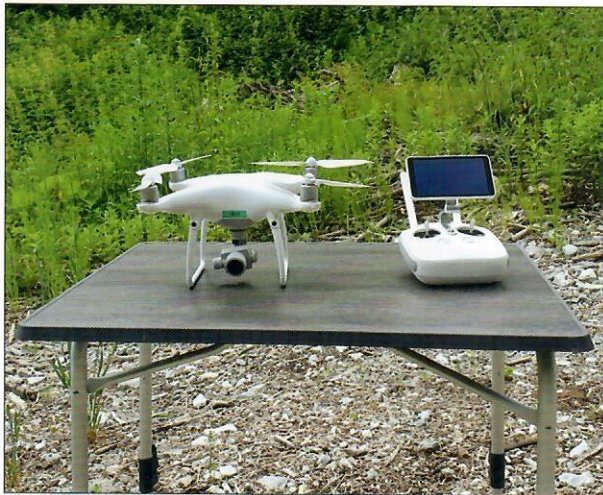
Obr. 2 Dron DJI Phantom 4 Pro
