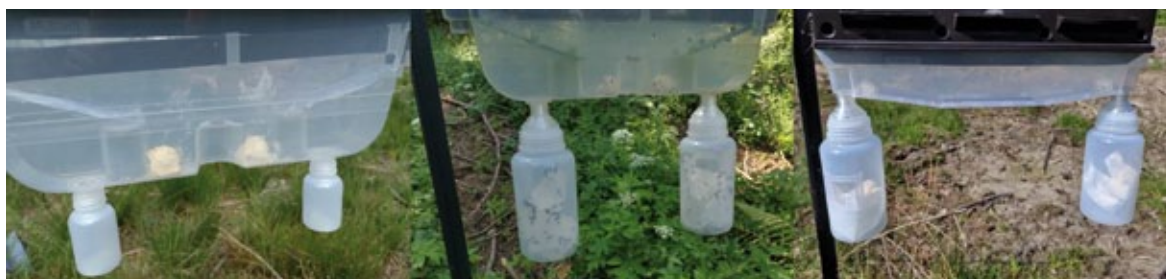
Obrázok 1. Upravená zberná vanička s nosičom huby B. bassiana . Roky z ľava do prava 2020, 2021, 2022 Figure 1. Modified collection tray with carrier of B. bassiana fungus. Years from left to right 2020, 2021, 2022
